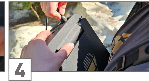
4 Lift the Control Unit to see the socket at the rear and plug in the probe.
