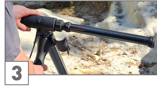
3 Unlock the probe mount clips and insert the Super Sensor in a comfortable height.
