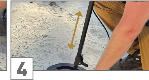
4 Adjust the Telescopic Rod to your body height to allow for more comfort while working with the detector. Lock the levers to fix the height.
