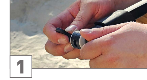
1 Unscrew the mounting screw from the coil mount at the Telescopic Rod. Make sure the rubber washers are seated next to the shaft before attaching the PentaCoil.
