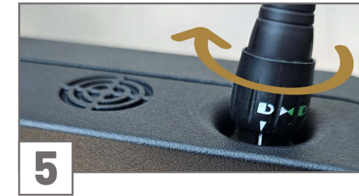
5 Align the white markings, push the plug into the socket, and rotate the plug cap clockwise to fix the plug.
