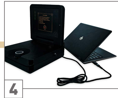
4 (1) Connect the Control Unit with the Windows notebook via USB-C cable.
