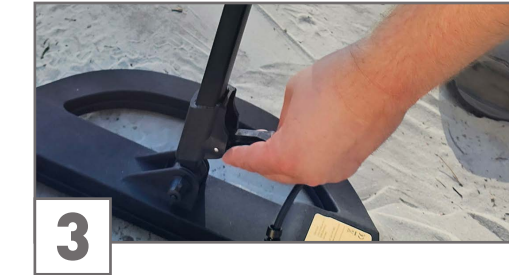
3 Use the locking levers to loosen the single segments of the Telescopic Rod.
