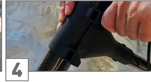
4 Lock the probe mount clips.
