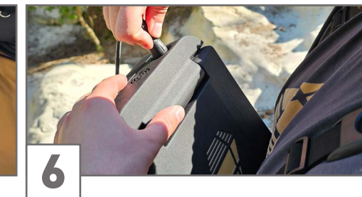
6 Plug the probe into the Control Unit – see 3.4 Backstrap + Control Unit on page 14.
