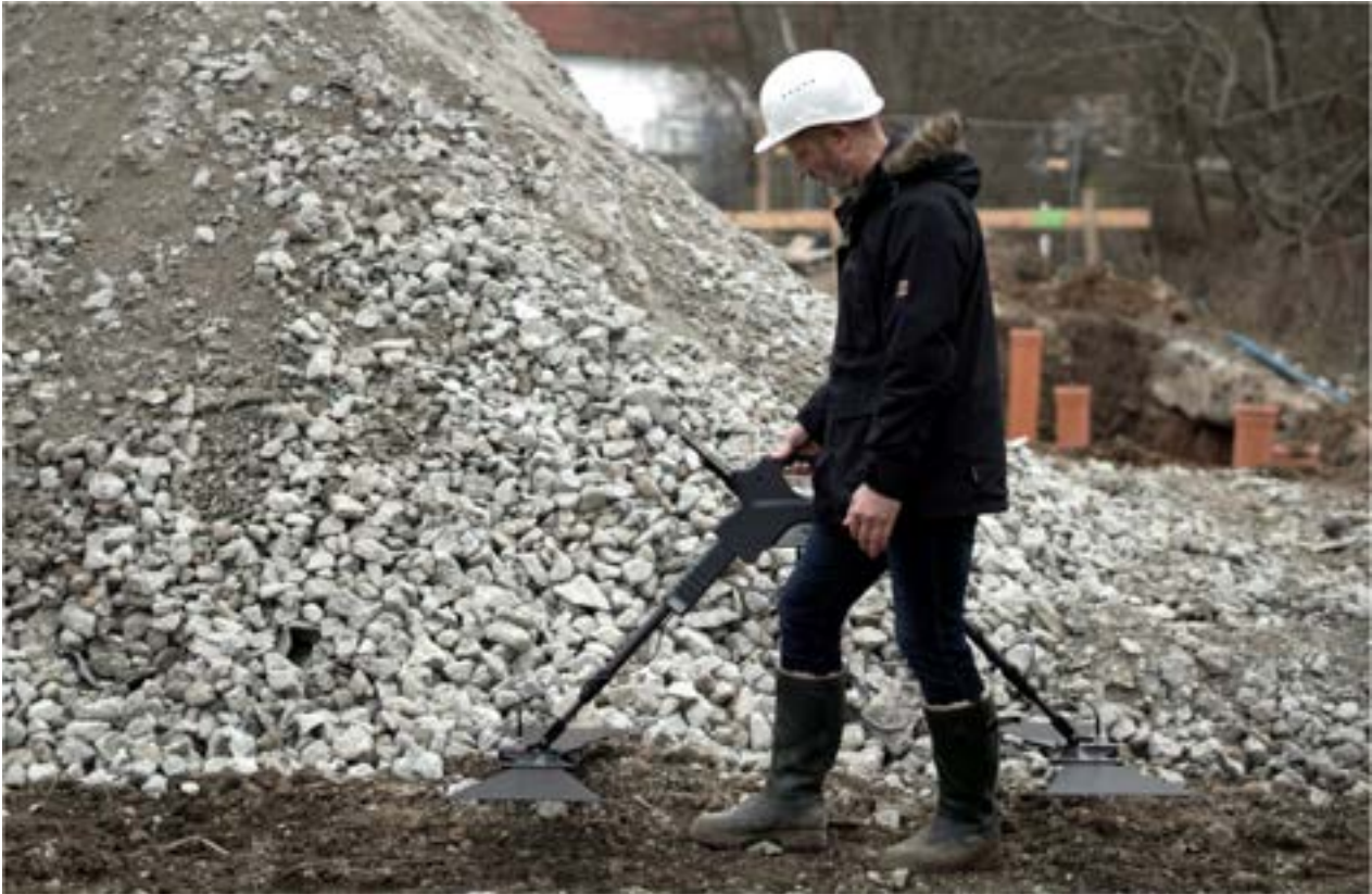
Figure 6.1: Holding the Gepard GPR before starting the scan
