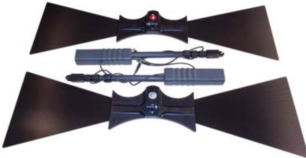
Figure 4.3: Triangular antennas with transmitter, receiver and telescopic shafts
